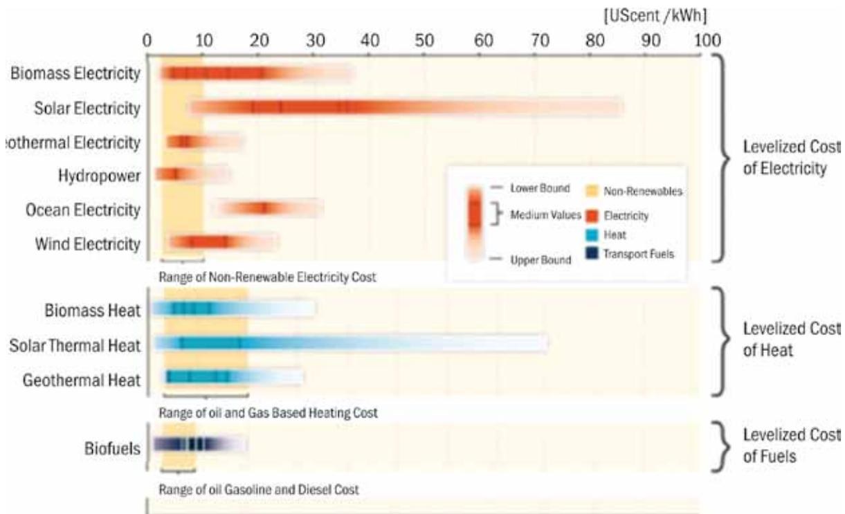
**Figure 4** Costs of electricity generated from various sources
