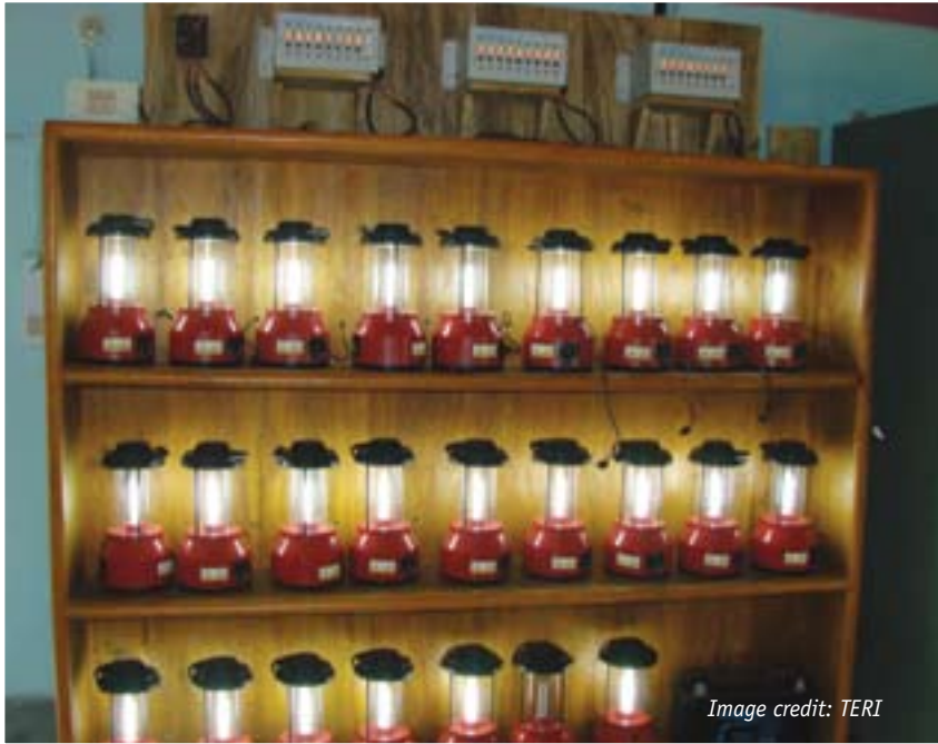
Solar lantern charging station
