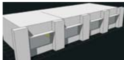
Recommended shading for southern façade
