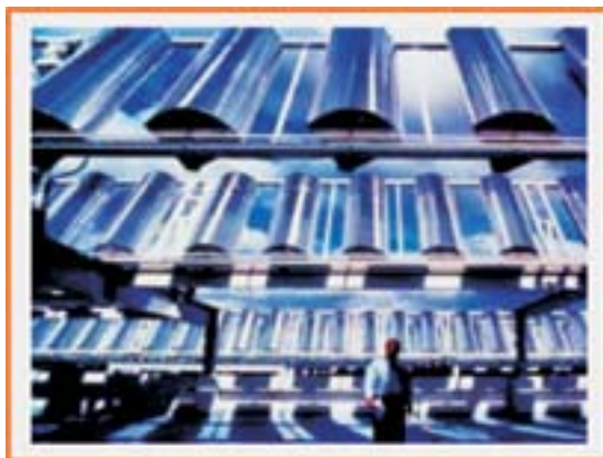
Figure 5 5200-sun, point-focus concentrator for a solar furnace. (Sandia National Laboratories/PIX01728)
