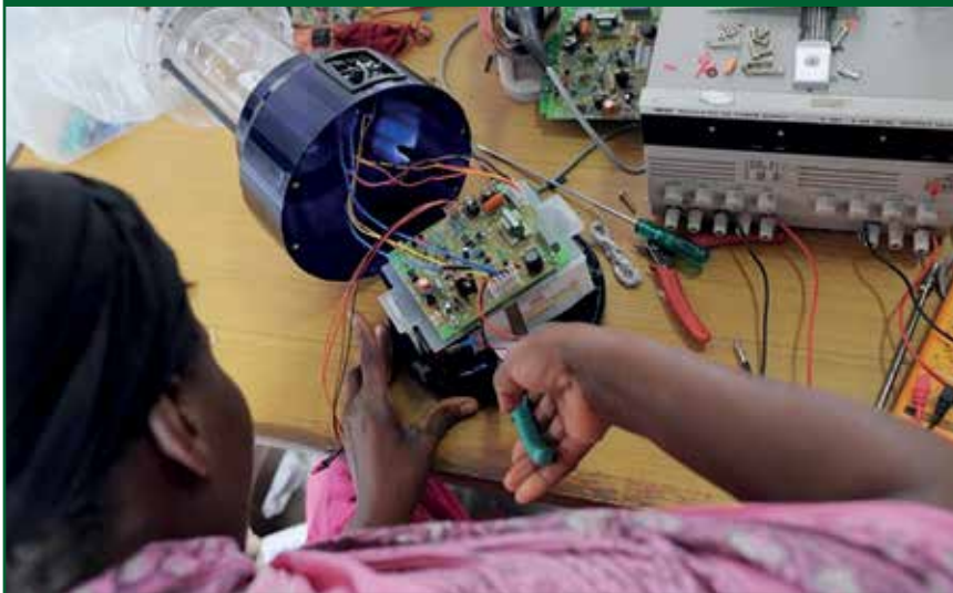
African Solar Mama learning how to fabricate charge controller
