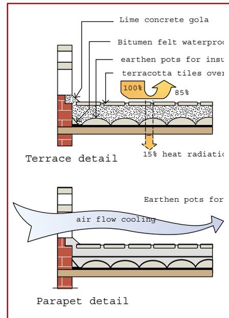
▲ Roof details showing use of earthen pots for roof insulation
