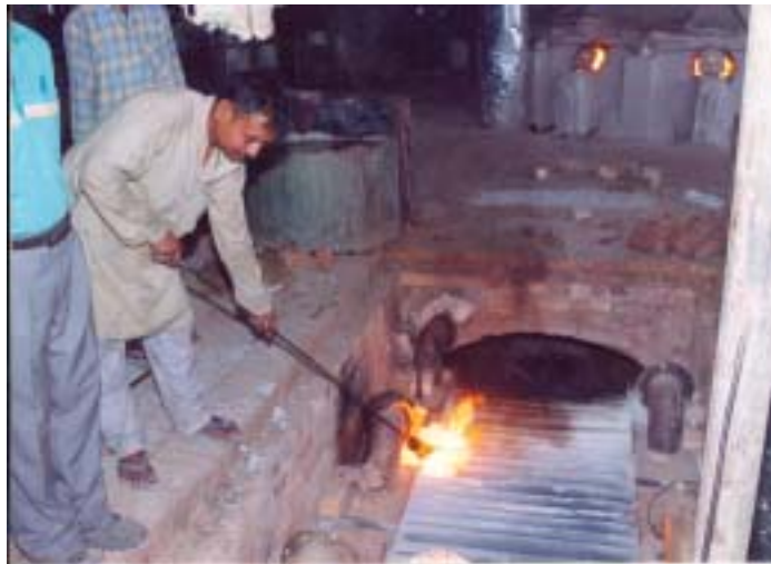
Figure 50 Testing for leakages with a palita
